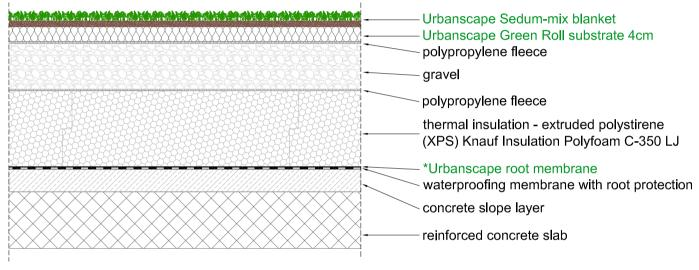
\* root membrane is recommended when waterproofing has no root protection
